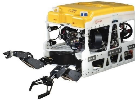
Figure 5-1: Example Light Work Class ROV SAAB COUGAR XT
